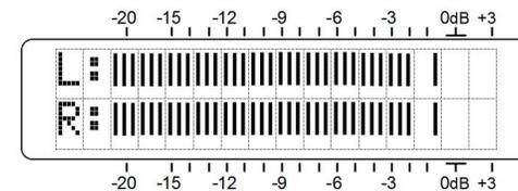
Although L and R (Left and Right) levels are shown here, the "stereo" outputs are simply for interconnect convenience, as most broadcast plants are wired for stereo whether the programming is or not. The two 634 outputs are the same, and the meters will indicate identical levels as well.
