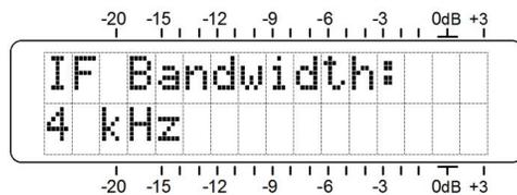
The frequency choices are 6kHz, 4kHz, 3kHz and 2kHz. These are the approximate -6dB points in each case, with a very precipitous drop above the turnover frequencies as shown below.
