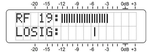
During normal receiver operation, whenever the `RF` bargraph falls below the tic mark, `LOW SIGNAL` will flash on the LCD screen and a carrier-loss alarm will be sent to the rear-panel connector. The rear-panel C (carrier-loss) terminal gives an NPN transistor saturation to ground on this alarm, which may be used to actuate a relay, light a remote LED indicator or tie into a remote control system.
